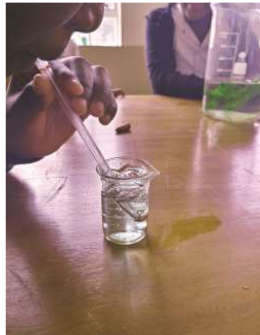
b. The bromothymol blue solution changes colour due to the acidic CO 2 found in exhaled air.
